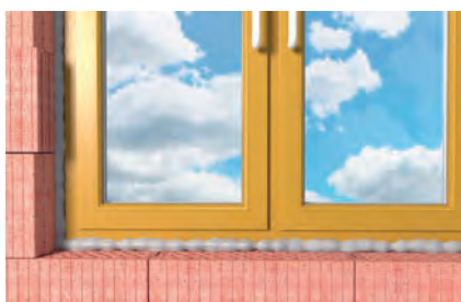
Window connection joints
