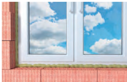
Window connection joints
