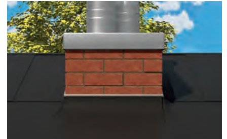
Sealings around roofs with bitumen sheeting
