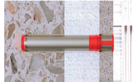
Detail: Repairing weather shells
